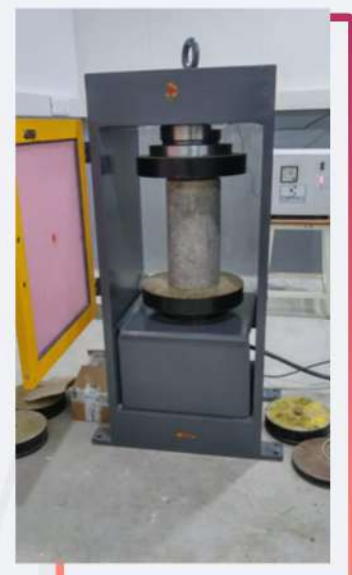
Fig. 3. Compression Testing Machine (3000kN)
