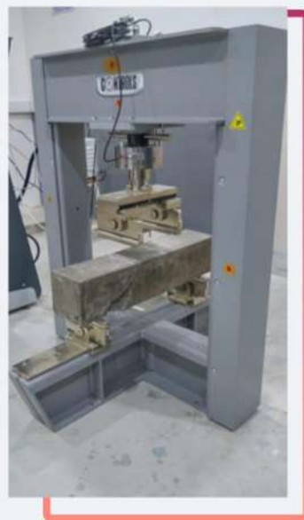
Fig. 2. Flexural Testing Machine (200kN)
