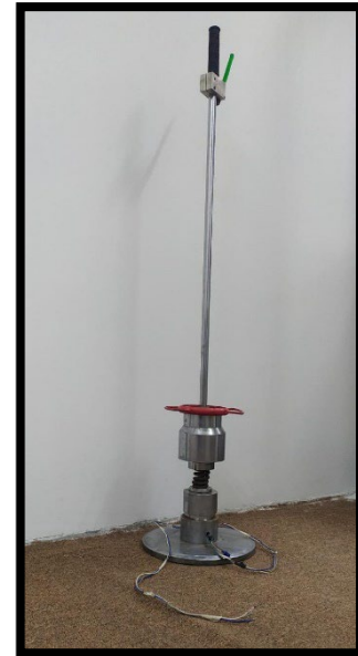
Fig. 2. Schematic diagram and photograph of LWD device
